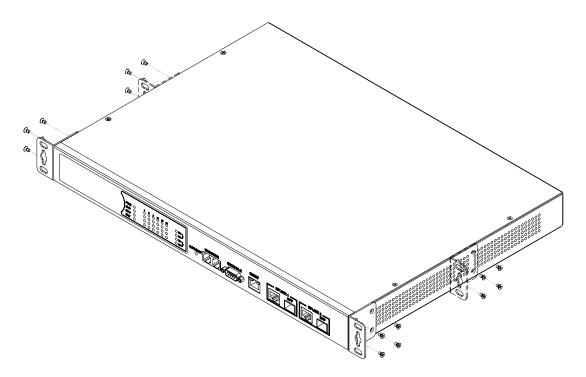
Figure 4-1. Attaching the Brackets
